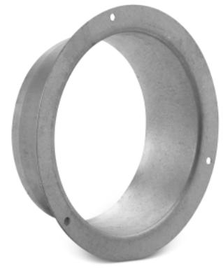
Circular mounting frame suitable for supply and exhaust air valves. Has three pre-cut holes for secure mounting on the ceiling. The frame is bent for easy insertion into spiral tubes.
