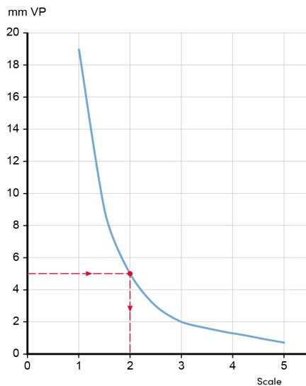
If a Pascal-based measuring instrument is used, divide by 10 (10 Pa = 1mm of water column)
