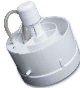
Sirrus KFS 125 is an all-Swedish invention which makes it possible to connect any type of cooker hood – regardless of the brand – to a mechanical ventilation system. A built-in pressure switch detects when the cooker hood is on and then opens from the set basic position to controlled forced operation (opening time approx. 30 seconds).
