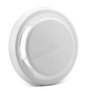
OPK is a round valve with aerodynamically design with good characteristics in terms of noise level, air flow capacity and pressure drop. The valve is mounted in a ceiling or a wall and is intended for ventilation systems with a relatively low pressure drop. The design of the valve and a gasket of moltoprene prevents soiling.
